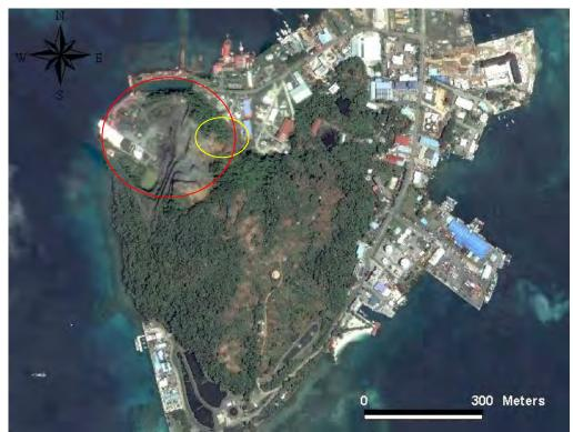
Figure 11 Malakal Island showing basalt quarry area (66,282 m²) marked in red circle which was once forest. An area of chronic landslides is circled in yellow that crushed an adjacent warehouse downslope after heavy rains in 2009. The area of slope failure has 70% slopes. Quarry activity has left a thin and unstable rim of steep sloped forests that has caused several landslides after heavy rains. Source: PALARIS 2006 Mikonos Satellite Imagery.
