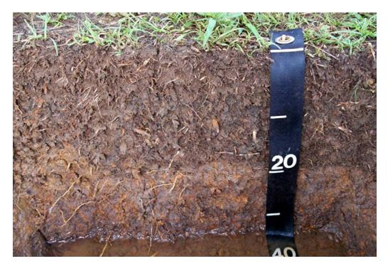
Figure 29.—Profile of Dechel silty clay, 0 to 2 percent slopes (map unit 616). This is a bottom-land soil with a high water table. Wet soil conditions are indicated by the gray soil matrix and the oxidized (rust-colored) root channels. This site is in the Ngerikiil Valley, Airai State, Babeldaob Island.
