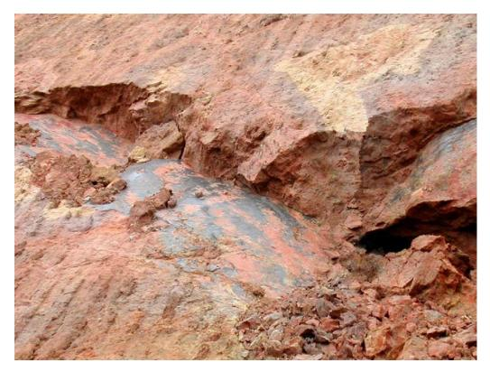
Figure 26.—Fracture planes characterized by smooth surfaces commonly coated with a red and black sheen (iron and manganese) are randomly oriented in the volcanic rocks on Babeldaob Island. In this photo, two fracture planes meet at a right angle. Removing supporting soil where a fracture plane is oriented downhill is likely to increase the risk of slumping. The vertical exposure in the center of the photo is about 1 meter high.
