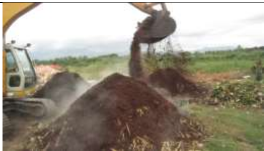
Photo showing wood chips used as cover, moisture control and source of carbon for market waste composting
