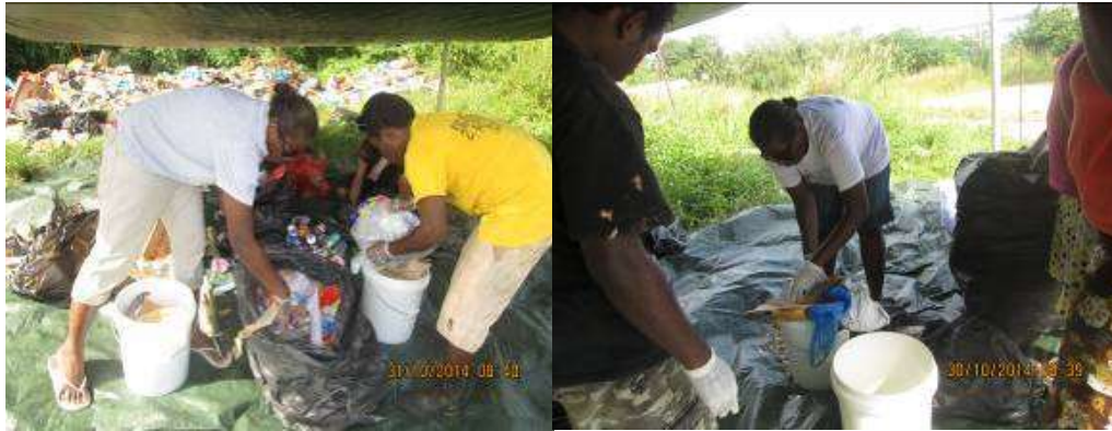
Photo 5: Measuring the density of the waste by transferring all the collected waste into a bin
