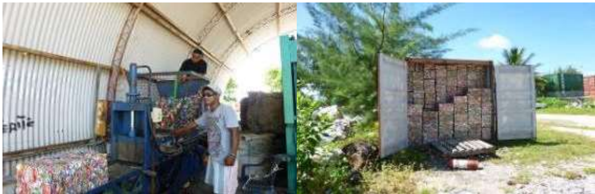
Baling and processing of aluminium cans for export in Tarawa, Kiribati
