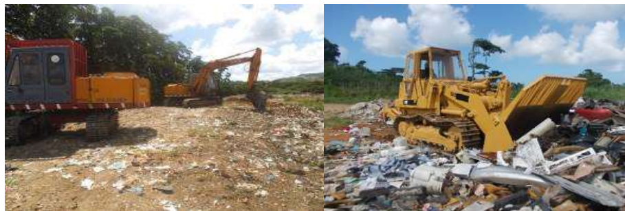
Bulldozer (right) and excavator (left) are the main equipment for waste landfill operations
