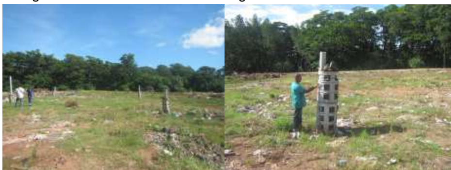
Measuring the temperature at one of the gas ventilators at the Labasa Landfill, Fiji
