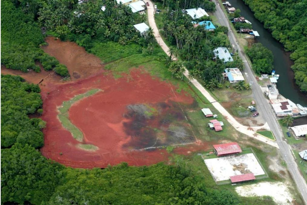
Figure 15.—An area of Orthents-Urban land complex, 0 to 50 percent slopes, which is densely covered with buildings and other impermeable surfaces or has been highly modified by earth-moving activities. The bare soil indicates the difficulty in revegetating disturbed volcanic soils. This area is located in Ngaremlengui State, Babeldaob Island. Photo courtesy of Dr. Pat Colin, Coral Reef Research Foundation.
