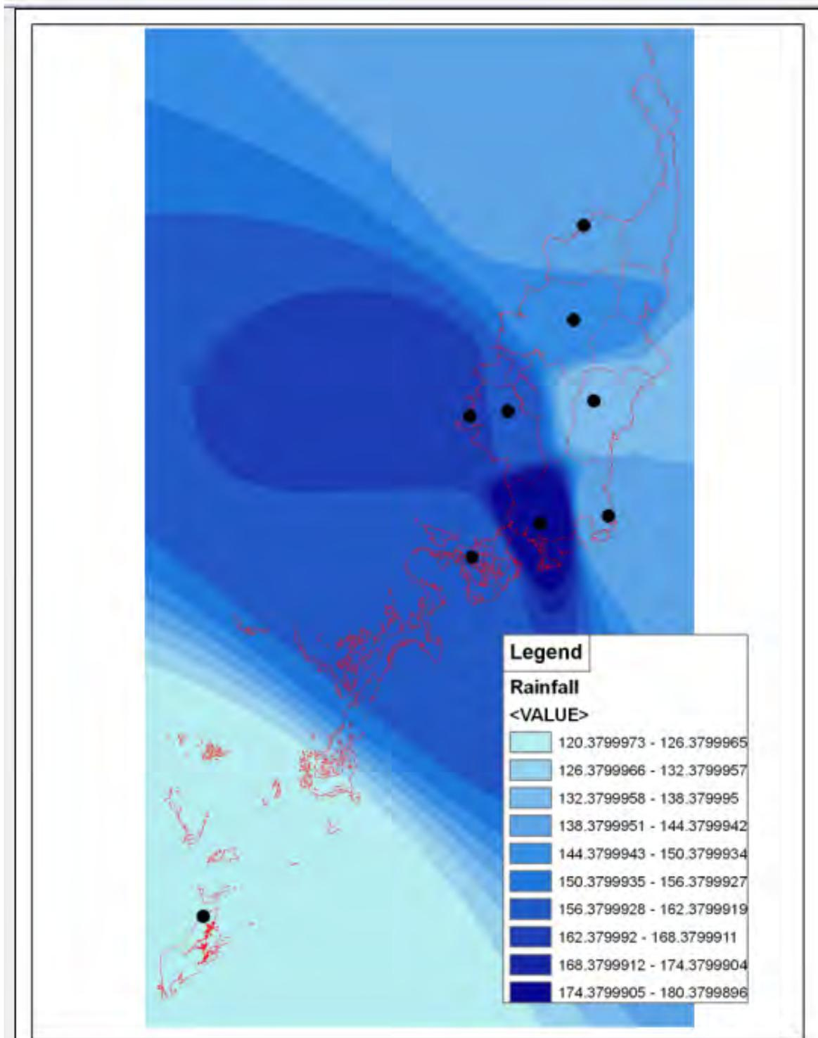
Figure 3 Annual Precipitation Map for Palau (inches/year) showing location of rain gages as black dots
