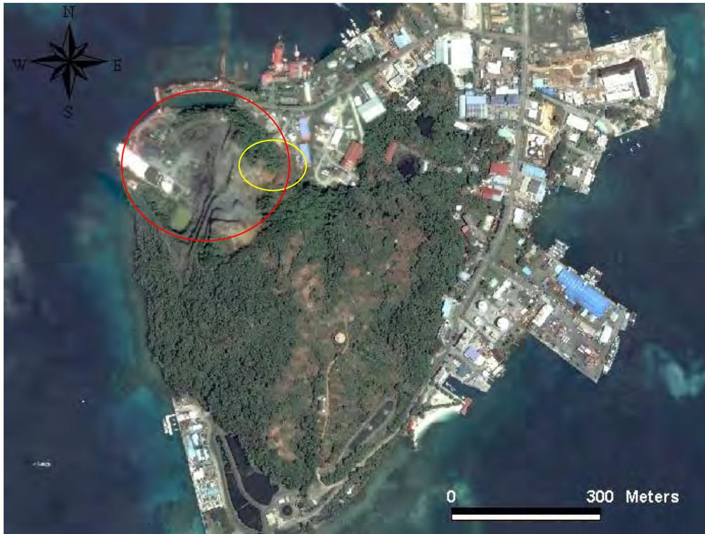
Figure 11 Malakal Island showing basalt quarry area (66,282 m<sup>2</sup>) marked in red circle which was once forest. An area of chronic landslides is circled in yellow that crushed an adjacent warehouse downslope after heavy rains in 2009. The area of slope failure has 70% slopes. Quarry activity has left a thin and unstable rim of steep sloped forests that has caused several landslides after heavy rains. Source: PALARIS 2006 Mikonos Satellite Imagery.
